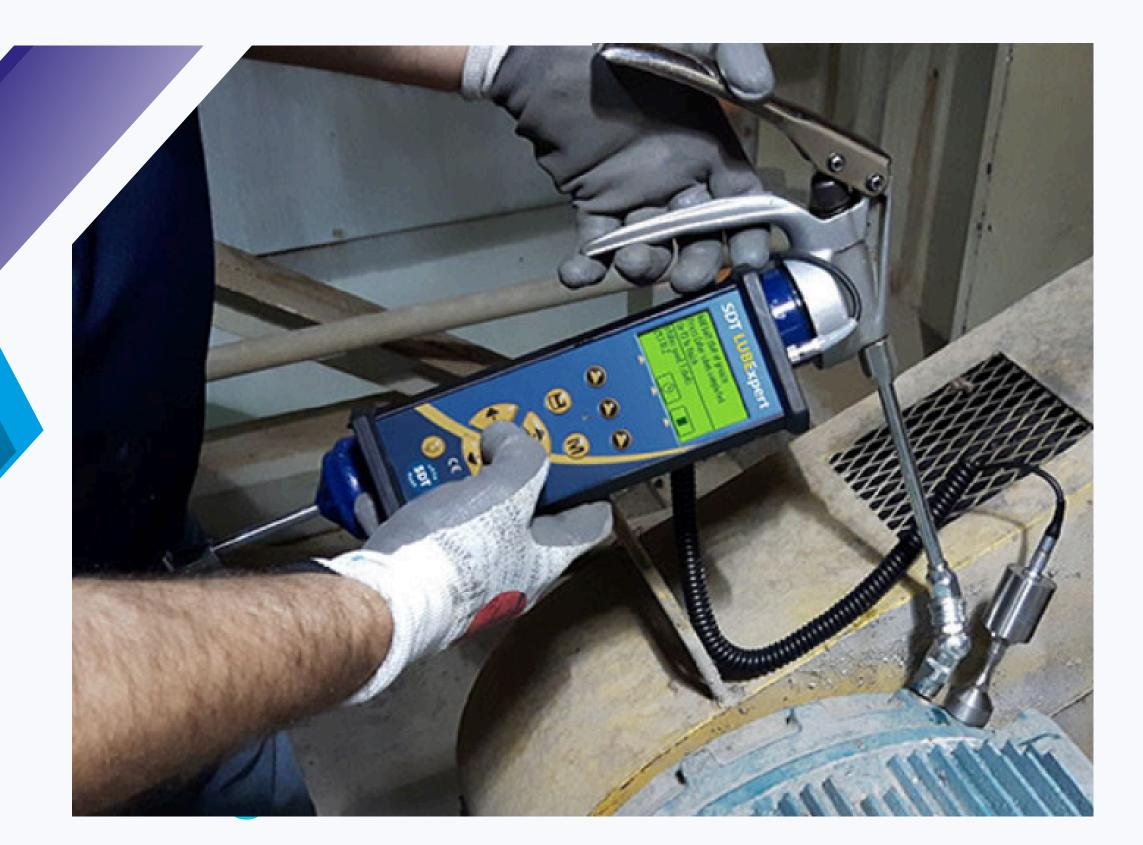
Ultrasound is the process of assessing the health and condition of your equipment by collecting and analysing ultrasonic signals produced during operation. It allows us to listen and interpret frequencies above the range of the human ear (above 20KHZ).
