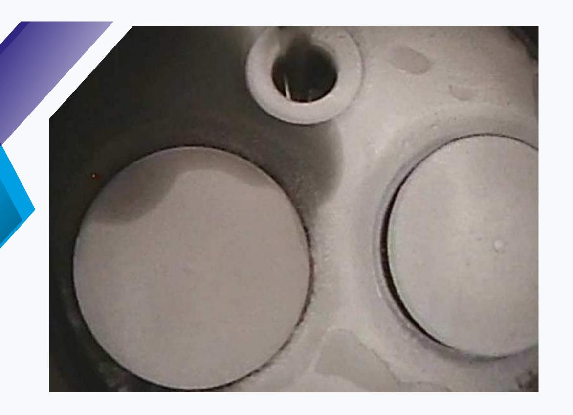
Borescope inspection is a costeffective, non-invasive method to assess the internal condition of a generator's combustion chamber, enhancing safety, reducing environmental impact, and ensuring equipment reliability by identifying and addressing potential issues efficiently.
