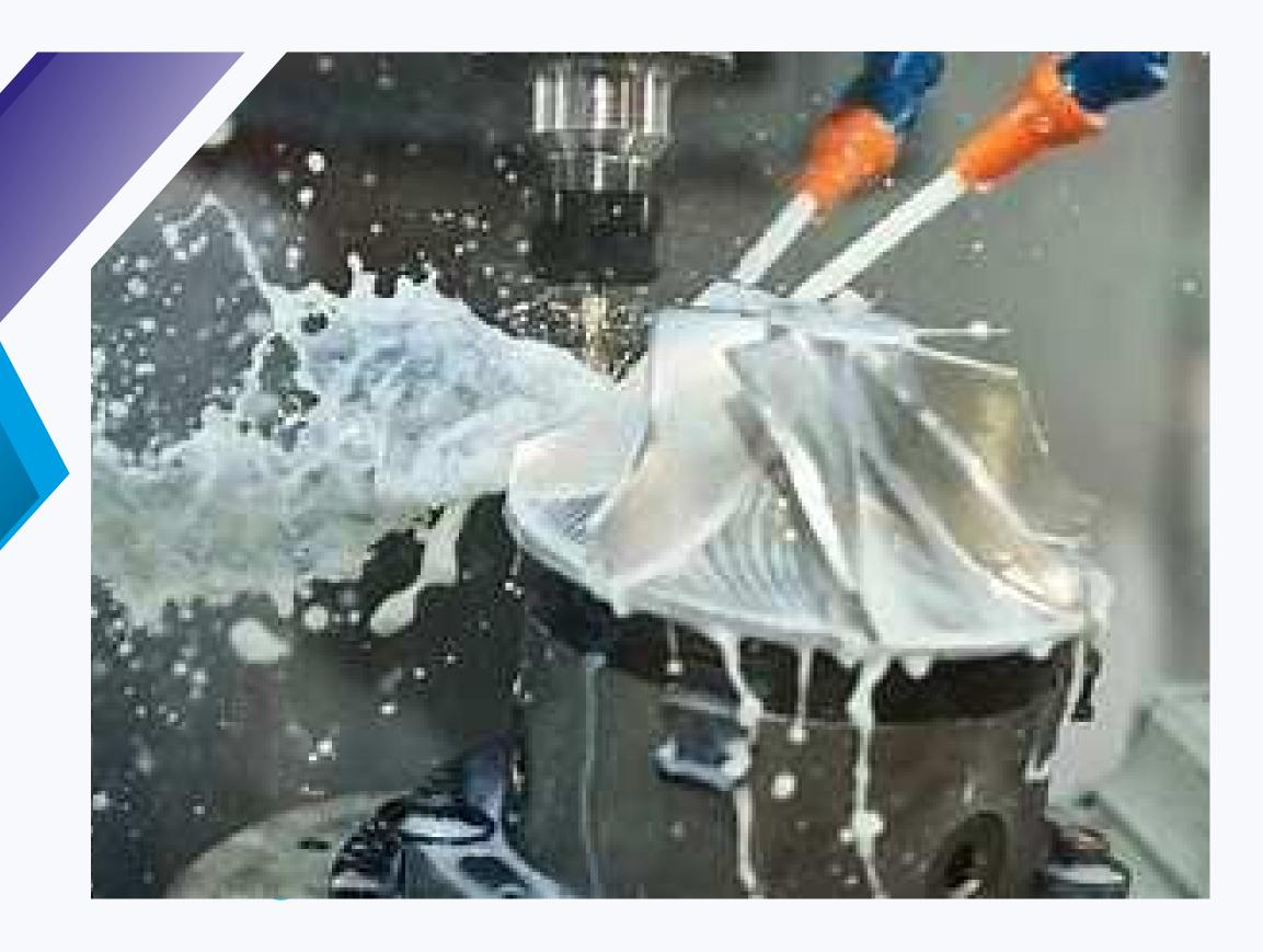
Pure Fluid Care involves the ongoing management and maintenance of metal working fluids by testing coolant concentration, pH levels, sump temperature and monitoring bacterial growth.
